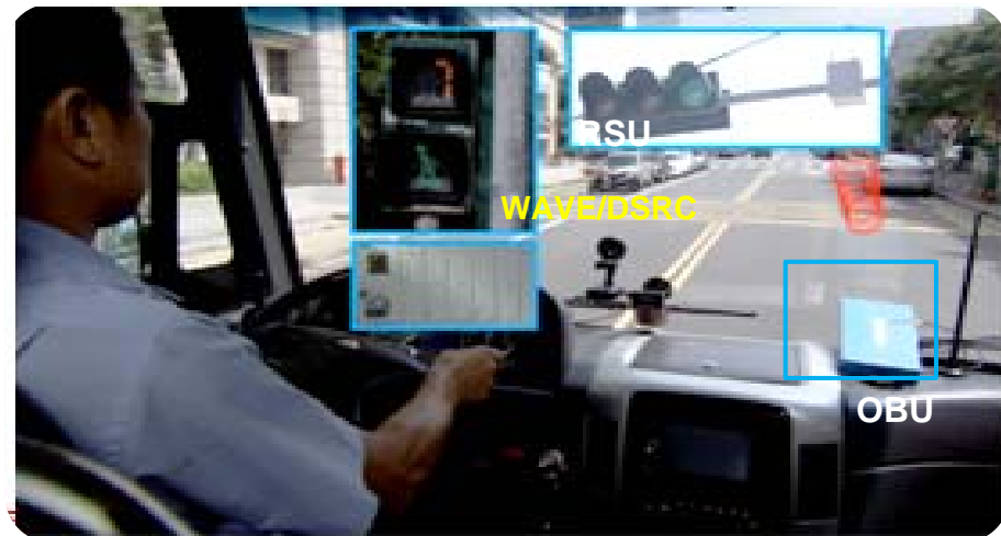
ITRI OBU Deployment on the Transit Bus
