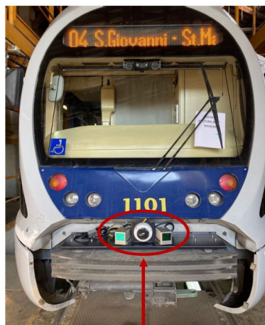
Mono camera and Long Range Front Lidars: LIVOX HORIZON
